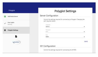
The user interface is designed to be simple and intuitive to use. Pictured above is the settings page. Using the menu bar on the left, new node servers can be added and existing node servers may be monitored. The button on the bottom of the menu will open Polyglot's log in a new browser window.
