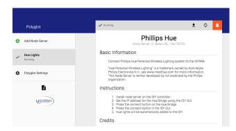
Clicking a Node Server in the menu will activate the node server view. In this view, there is a menu bar at the top. This menu bar will indicate is the node server is Running or Stopped. It also provides buttons to download the profile, restart the node server, or delete the node server.
